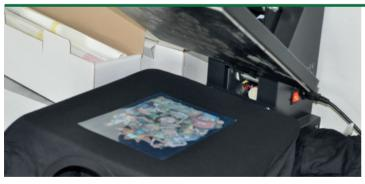
PLACE THE GRAPHIC ON THE T-SHIRT, HEAT-PRESS IT AND AFTER REMOVE THE POLYESTER CARRIER
